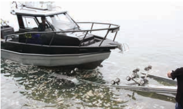
Straps removed, bung is in, engine starts and ready to roll down the boat ramp.
